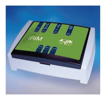
The IRiM (infra-red interface modul) uses modern infra-red technology to transmit measurement data from the AL400 photometer to one of 3 optional interfaces. These interfaces can be used to connect to a PC, a USB printer¹) or alternative a serial printer²). The interface which is selected is displayed by an LED function indicator. The user can switch between the interfaces using the "Select" button.
