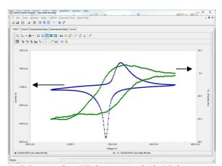
In Echem Analyst, I/E data are overlaid with frequency data as part of the standard data analysis. The chart selector gives the user flexibility to arrange charts in any number of ways.
