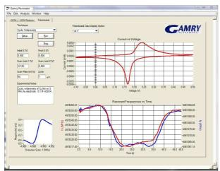
Frequency data are also displayed on the potentiostat tab during acquisition. Here are both the QCM and potentiostat responses during the cycling of a Cu film on an Au electrode.
